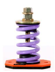
This unique range of open spring mounting uses an integral rubber end fixing of the spring which sets them apart from all other designs. Loose springs and plates are now history and high frequency and noise attenuation is provided regardless of whether rubber seating pad is used or not.
