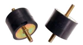
**Easyflex** Type EFRO mounts are very versatile and can be ideal for a wide range of applications where simple and compact anti-vibration mountings are required. They are suitable for loads in shear, as well as in compression. These mounts are used in an extensive range of applications including compressors, generators, air conditioners, pumps, fans, motors, laboratory equipment, scales, etc.
