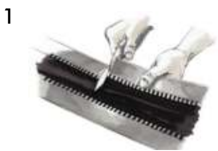
At a notch, cut a length equivalent to the perimeter required plus an overlap of 5 to 6 cm (2") for joining
