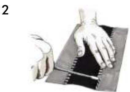
Lift the seam outwards at right angle
