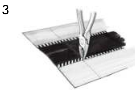
Make a cut at the edge of the lifted seam section
